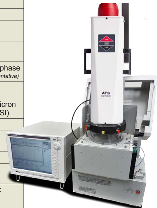
ThermoStream docked with enclosure
